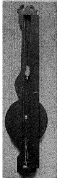
Fig. 32b. Back, open, showing the long tube of the barometer and the short tube with float counterpoised over the central pinion.
