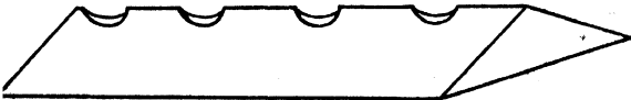
Fig. 9i.—Rest for Platinum needle and Platinum loop. Prevents contact of platinum with surface of table.
