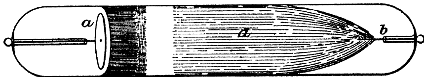
FIG. 1.—Electric discharge at a moderately low pressure. The negative electrode a is a disk, and is separated by a small dark interval from the blue negative glow e . The glow along the rest of the tube to the anode b is, in air, a diffuse band of reddish light, d .
