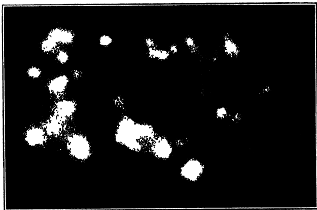
FIG. 15.—Photographic action of crystals of the mineral thorionite ( \beta and \gamma rays). Exposed 7 days.
