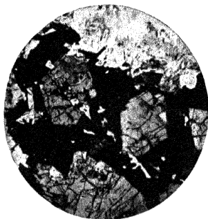
3.—Epidote. Ordinary Light. Showing form and cleavage.
