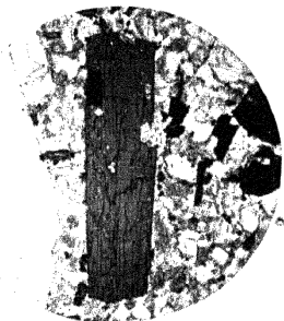
3.—Hornblende, vertical section. Ord. L. Showing form and cleavage.
