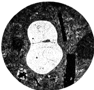
4.—Quartz. Ordinary Light. Showing corrosion.
