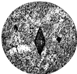
4.—Sphene. Ordinary Light. Showing form and high refractive index.
