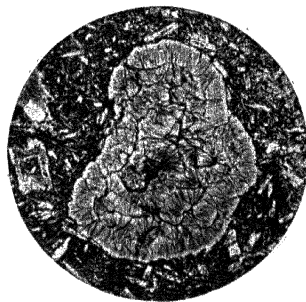
6.—Chlorite. Ord. L. Showing vermicular habit and occurrence in amygdale.
