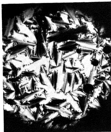
FIG. 26.—ETHYL ANISALAMINOCINNAMATE SHOWING THE FAN STRUCTURE OF THE SMECTIC TYPE. MAGNIFICATION ABOUT 18 DIAMETERS ( after Friedel ).
