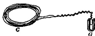
FIG. 91. — Circuit arranged to show the phenomena of induced currents.
