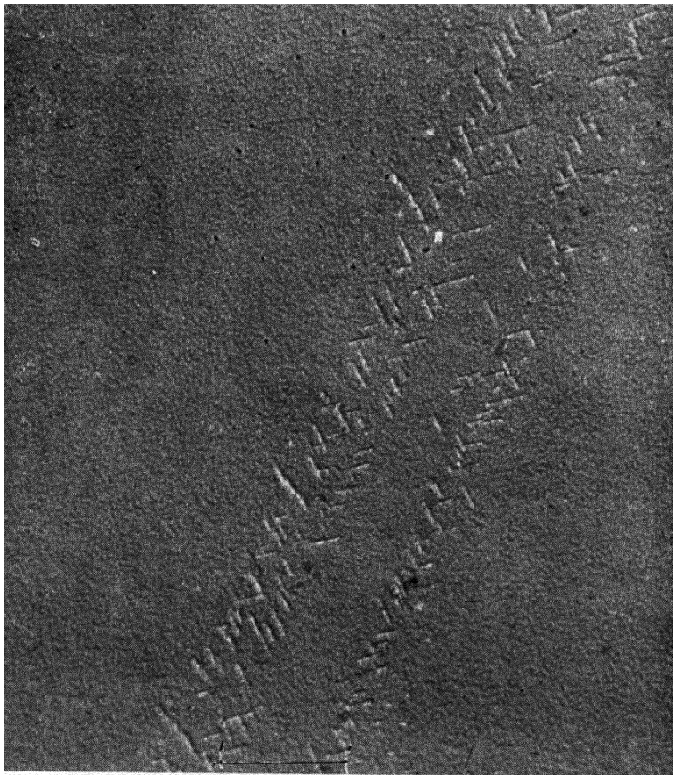
Fig. 32. Precipitation along a slip band in an aluminium-4-per-cent-copper alloy aged 3 hr at 190^{\circ}\text{C} . (106), (107) ( \times 25,000 )
