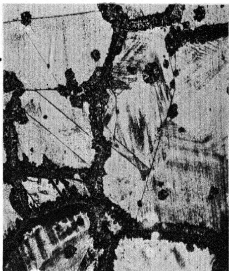
Fig. 34. Typical discontinuous precipitation starting from grain boundaries in a copper-1.97-per-cent-beryllium-0.03-per-cent-iron alloy aged 2 hr at 325°C. (2) ( \times 75 )
