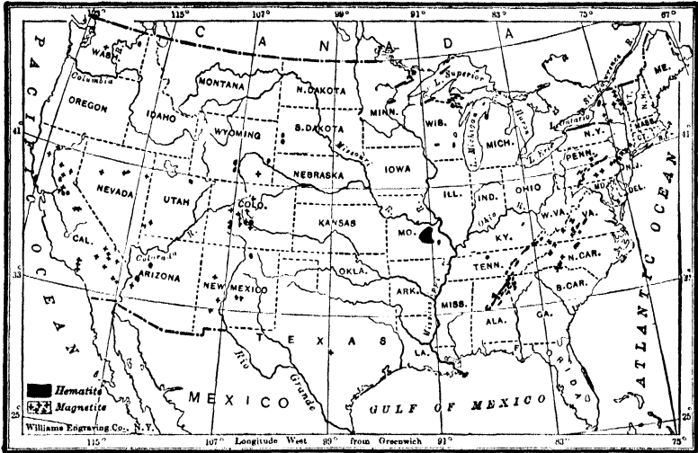
FIG. 226. — Map showing distribution of hematite and magnetite in the United States. (After Harder, U. S. Geol. Survey, Min. Res., 1907.)
