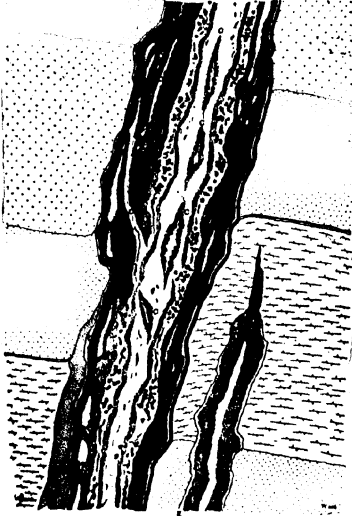
FIG. 215. — Vein filling a fault fissure. Enterprise mine, Rico, Col. (After Rickard, Amer. Inst. Min. Engrs., XXVI, 1897.) Shows irregular banding, also vugs in center of vein. White vein material is quartz; dark, is blende and rhodochrosite.
