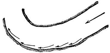
FIG. 127. — River curve indicating place of greatest erosion, on bend. (Thomas and Watt.)
