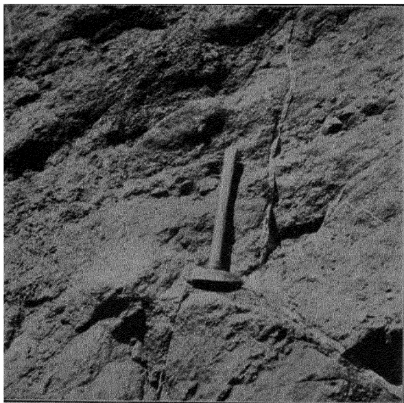
FIG. 196 f . — Soft conglomerate with gypsum seams. Foundation rock of part of the St. Francis dam. (H. Ries, photo.)
