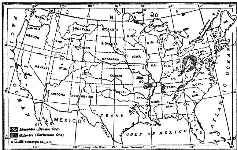
FIG. 227.— Map showing distribution of limonite and siderite in the United States. (After Harder.)
