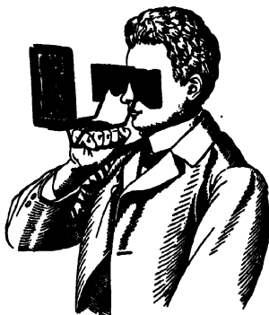
FIG. 10.—SHOWING METHOD OF USING THE VERANT VIEWER.
