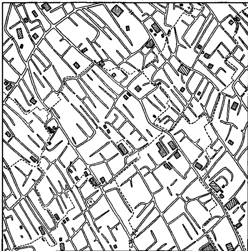
FIG. 139.—The canal system in one square mile of the delta southeast of Shanghai. The average distance between waterways is 380 ft., most of which are navigable. Footpaths are dotted and farm clusters ruled. One inch equals 1,220 ft. ( Whangpoo Conservancy Board. )
