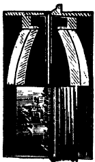
FIG. 31.—Ross's Wide-angle Symmetric Lens.
