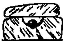
FIG. 18.—Black's Ice Calorimeter Experiment
