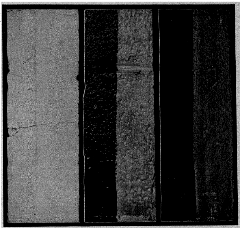
Panel No. 1. Entire surface primed with aluminum paint (var- nish vehicle) with 1 top coat white paint on right half.
