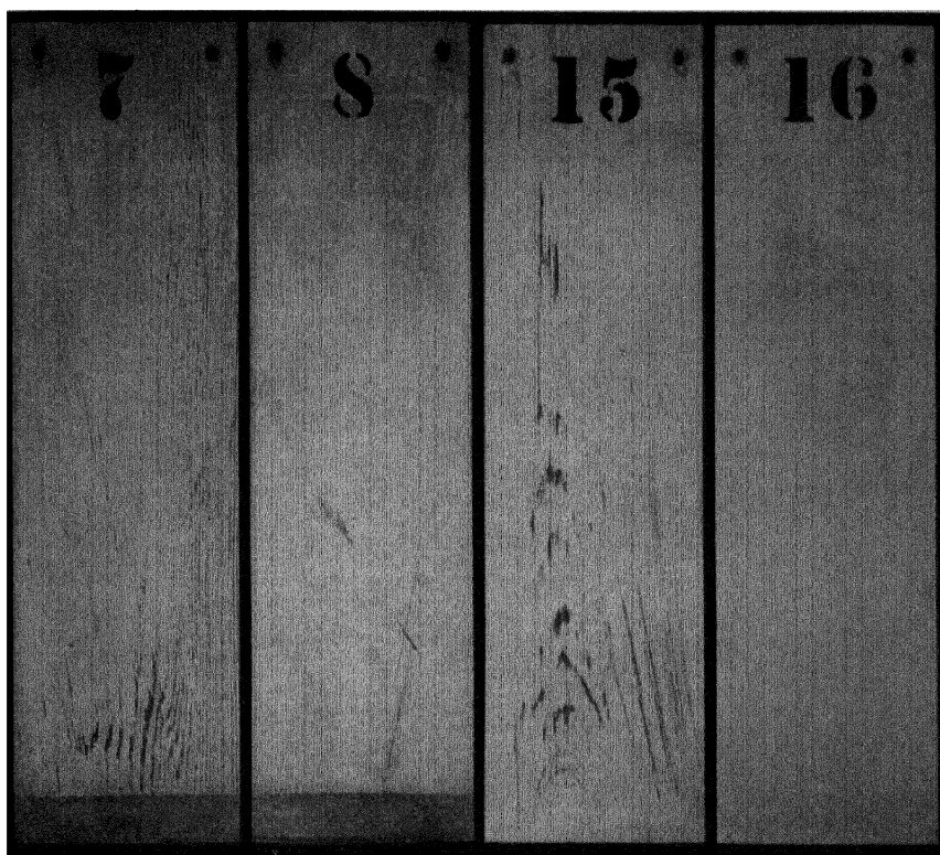
Panel No. 7. Yellow pine with 3 coats white lead paint. Panel No. 8. Yellow pine with 1 coat aluminum paint and 2 coats white lead. Panel No. 15. Cypress with 3 coats titanox-zinc oxide paint. Panel No. 16. Cypress with 1 coat aluminum paint and 2 coats titanox-zinc oxide paint.
