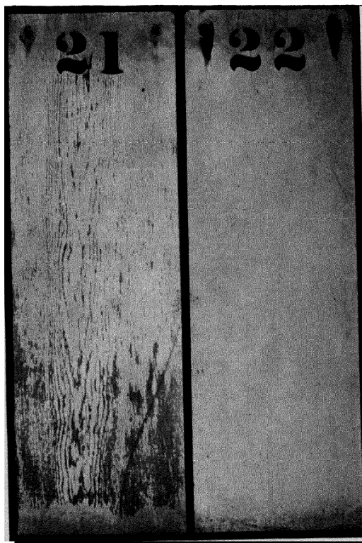
FIGURE 55. Appearance of wood test panels after 12 months' exposure at Washington. (Courtesy of H. A. Gardner.)
