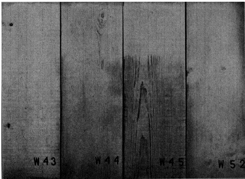
FIGURE 66. Western yellow pine with 2 coats of aluminum paint on lower portion and 3 coats above, after 44 months' exposure at New Kensington; aluminum paint made with 80-gallon ester gum varnish (No. 43), 50-gallon ester gum varnish (No. 44), 40-gallon ester gum varnish (No. 45), kettle-bodied linseed oil (No. 52).
