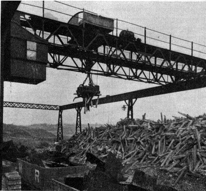
FIG. 240.—WITTON-KRAMER CIRCULAR LIFTING MAGNET ON OVERHEAD TRAVELLING CRANE, HANDLING PIG-IRON. (By courtesy of Witton-Kramer Works.)
