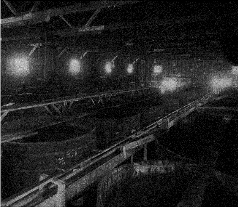
FIG. 37.—Redwood tanks. 17,000-25,000 gallons capacity. (Courtesy of the American Wine and Liquor Journal, New York.)
