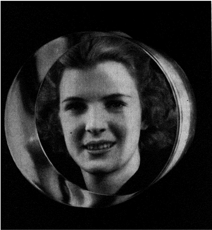
FIGURE 54. Transparency is a relative term. The nine and a half inch thickness of Lucite through which this subject was photographed is seen to be highly transparent to visible light, whose wave-lengths range from 400 to nearly 800 milli-microns. Advance information indicates that at 350 milli-microns (ultraviolet) about 75 percent of the radiation is transmitted by a 1-inch thickness; at 302 milli-microns, about 1 percent. (Courtesy E. I. du Pont de Nemours & Co., Inc.)
