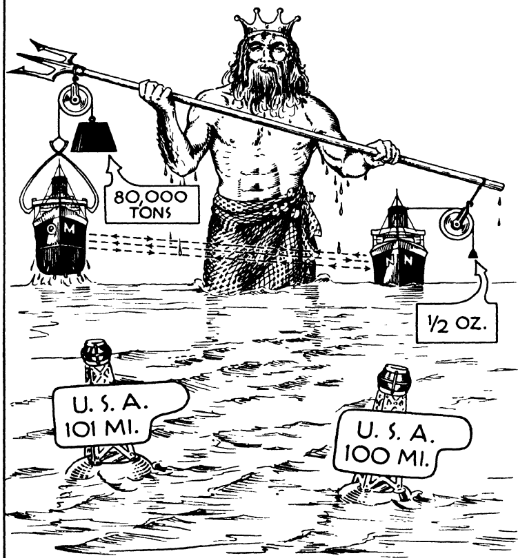
FIGURE 5. The weight of the half-ounce mass hanging over one of Father Neptune's pulleys counterbalances the Queen Mary's attraction for the Normandie.
