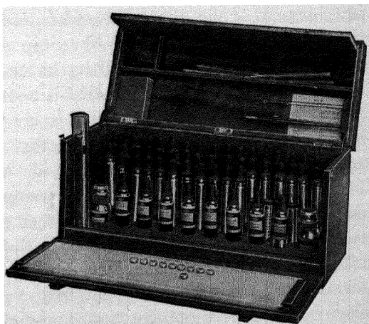
FIG. 47. — LaMotte Hydrogen-Ion Testing Set (Model 5B). A single test can be made in a few seconds. Only one drop of material is needed for a test. Results are accurate to 0.1 pH .
