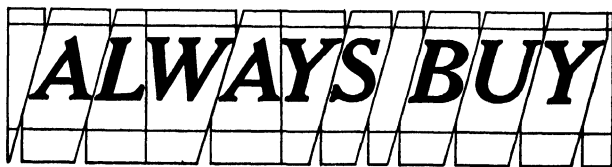
Fig. 95. Intertype Display Italic Matrices are of a special angular-cut design which makes it possible to fit the characters closely together. When the matrices are assembled, the angular cuts dovetail and the matrix characters are located properly with respect to each other. The precise spacing and proportion of characters demanded for advertising composition and other classes of display work are thereby obtained. Special opening and closing quads and hair spaces are provided for use with display italic matrices.
