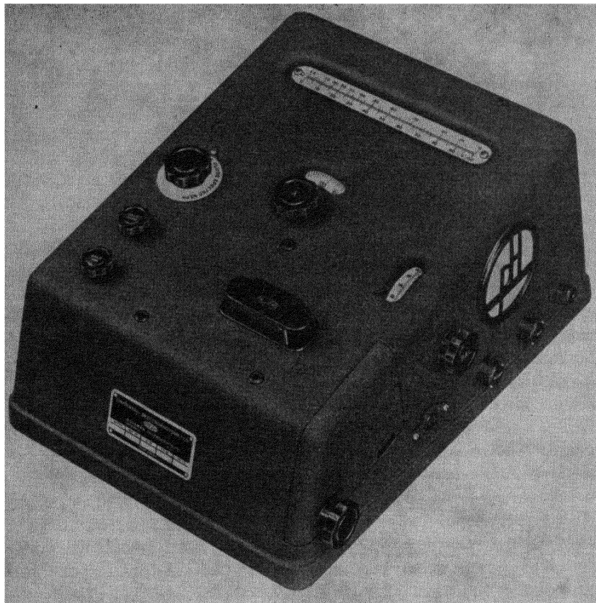
Fig. 17-13. Coleman replica grating absorption spectrophotometer, Universal model. (Photo courtesy Coleman Instruments, Inc., Maywood, Ill.)
