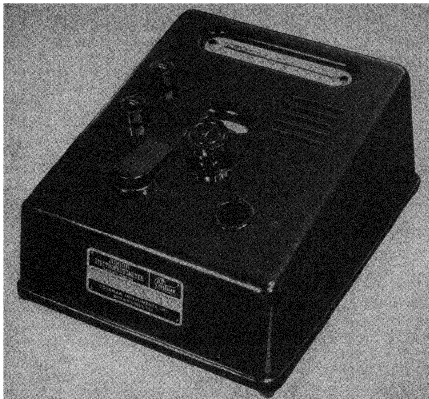
Fig. 17-10. Coleman Junior absorption spectrophotometer, used for colorimetric determinations in many soil testing laboratories. A replica grating gives a continuous series of wavelength bands from 400 to 700 m\mu (Fig. 17-14). (Photo courtesy Coleman Instruments, Inc., Maywood, Ill.)
