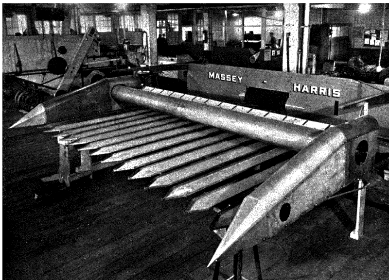
12 (a). Massey-Harris Combine 'comb' attachment as used for sunflower crops in America
