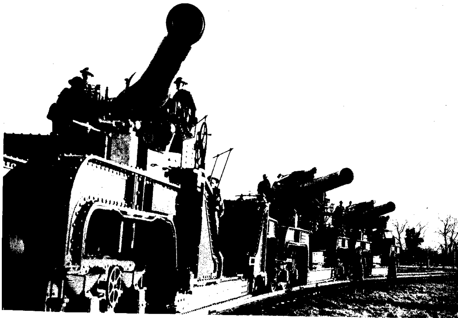
Howitzers to answer Hitler's invasion threat. The mighty weapons with which we shall withstand the projected Nazi assault. They are shown on their railway mountings, with barrels swung inboard ready for travel.
