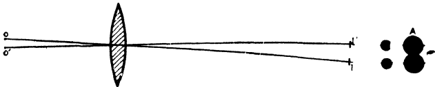
FIG. 22.—Diagram illustrating the effect of N.A. on resolution. The disc images I are shown in elevation on the right: at A are shown the larger disc images which would be produced by a lens of small N.A.
