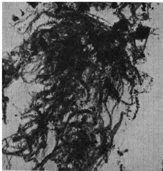
FIG. 205. ACTIVATED SLUDGE, SHOWING THE FILAMENTARY STRUCTURE OF THE AGGREGATES
