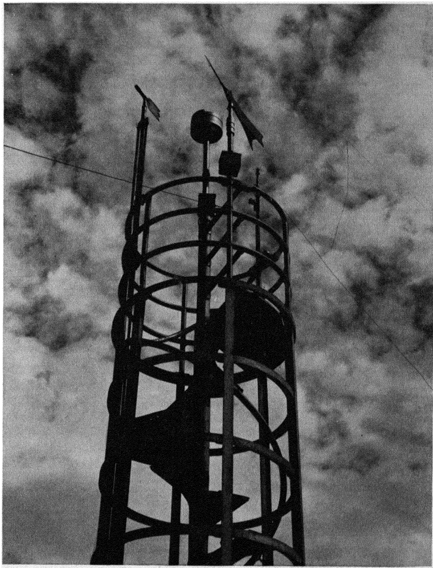
Fig. 15. Wind Instruments. These instruments are mounted on the tower support on top of the observatory of the central office of the U. S. Weather Bureau, Washington, D.C. From left to right, Dines (pressure tube) anemometer, thunderstorm indicator (generating voltmeters), 4-foot wind vane, and 3-cup anemometer. The anemometer is whirling quite rapidly so that the cups are not discernible. Courtesy, U. S. Weather Bureau and L. E. Johnson.
