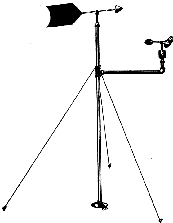
Fig. 45 Wind vane and anemometer on pipe-fitting support.
