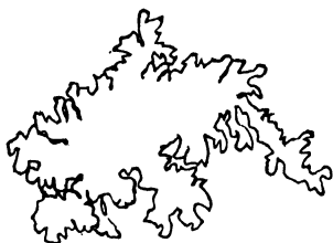
FIG. 3.—Metallic Iron in Sahara Sand, 100 : 1.
