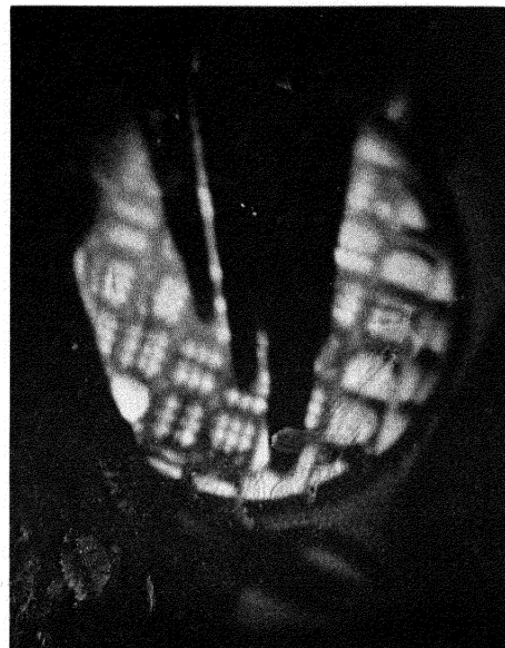
Figure 4. The phosphorescence of the core at 10 kw power level (photographed through a water-layer)
