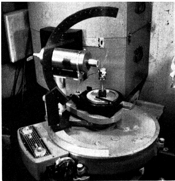
Figure 6. Neutron diffraction spectrometer for single crystals. Small high pressure \text{BF}_3 counter is adjustable on arc mounting added to GE X-ray unit. Sample crystal is \text{BaTiO}_3 .
