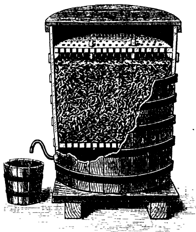
FIG. 28.— Quick vinegar process.
