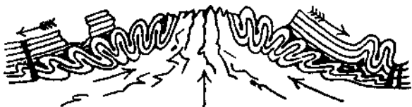
FIG. 14.—Section drawn by G. P. Scrope in 1825, to illustrate the effects of the upthrust of crystalline rocks through overlying stratified deposits, and the sliding and overfolding on the flanks of the resulting mountain-chain. The dykes shown in black are igneous intrusions spreading from the granite.
