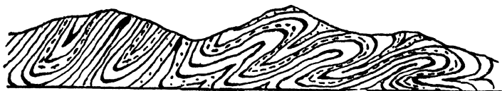
FIG. 150.—STEEPLY-INCLINED AND RECUMBENT FLEXURES.
