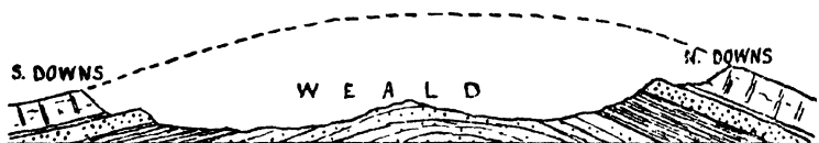
FIG. 159.—SECTION ACROSS THE WEALDEN AREA—A DENUED ANTICLINE.
