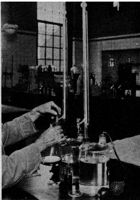
Fig 4 —DETERMINATION OF AMMONIA IN AMMONIACAL LIQUOR (4).
