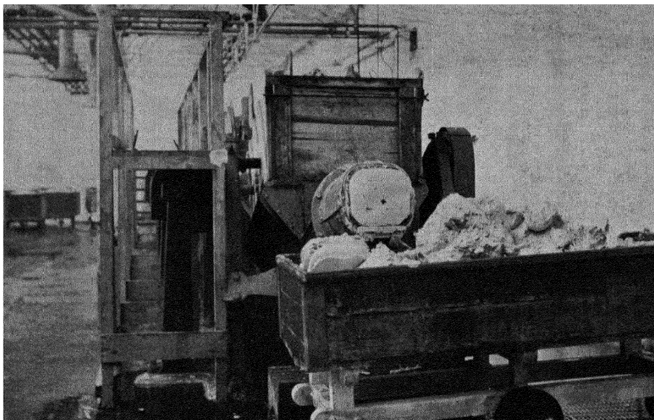
Fig. 2.—"MULTIPLEX" MARGARINE KNEADING MACHINE, SHOWING EXTRUSION END.
