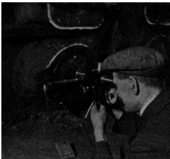
Fig. 6.—AN OPTICAL PYROMETER BEING USED TO READ THE TEMPERATURE OF A GAS RETORT.
