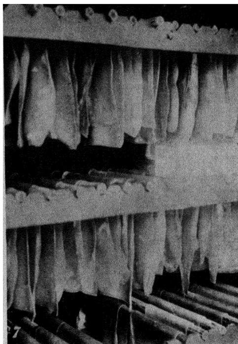
Fig 3—INTERIOR OF A "SMOKE HOUSE" Showing the sheets of rubber hung up to dry in the hot, smoky air provided by a wood fire.
