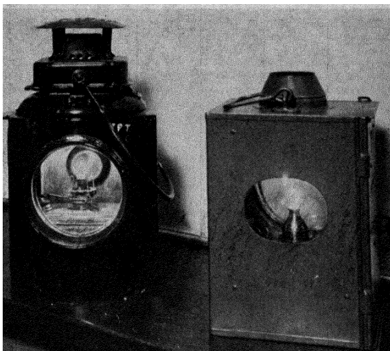
Fig. 4.—BURNING TESTS ON LONG TIME BURNING OILS. The photograph shows the standard types of lamp (Adlake on the left, Welch on the right) used for testing long time burning oils. In this case the test is prolonged for a seven-day period and the lamps are inspected each day.
