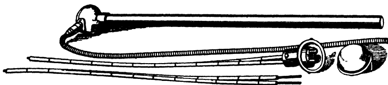
Fig. 2.—THE CONSTRUCTION OF A THERMOCOUPLE.
