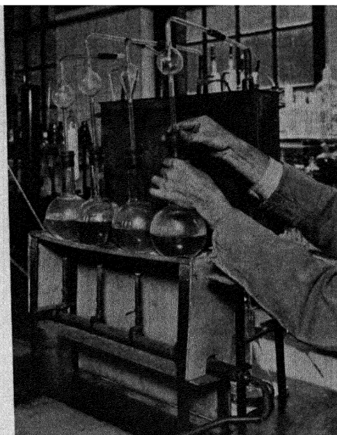
Fig. 2. —DETERMINATION OF AMMONIA IN AMMONIACAL LIQUOR (2). Inserting the splash head prior to distillation for 45 minutes.
