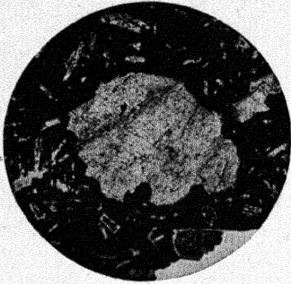
1. Calcite. Showing cleavages and the occurrence in amygdule.
