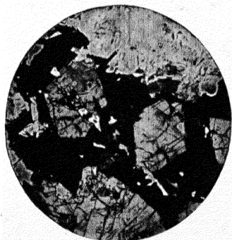
3. Epidote. Showing form and cleavage.
