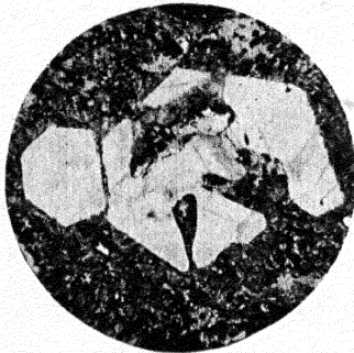
3. Quartz. Showing corrosion.
