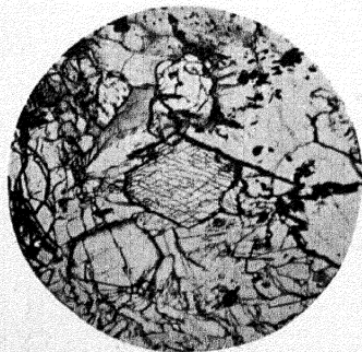
4. Glaucophane, trans. sect. Showing form and cleavages.
