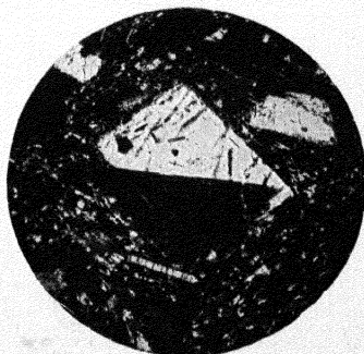
6. Sanidine. Crossed polarisers. Showing Baveno twinning.
