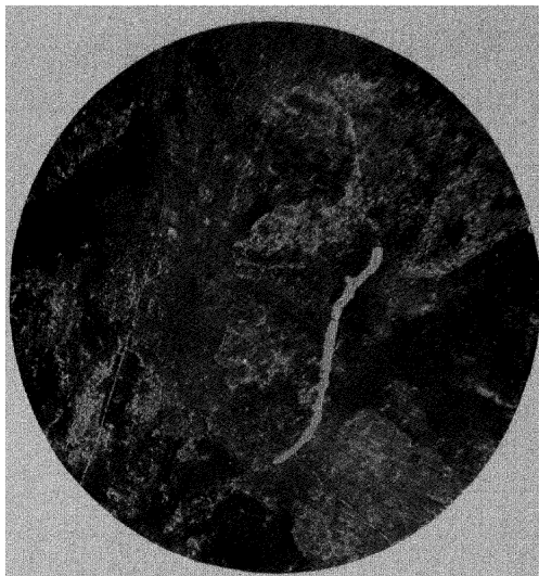
PHOT. 16.—“PEARLITE GRAINS” AND “FREE” FERRITE.
