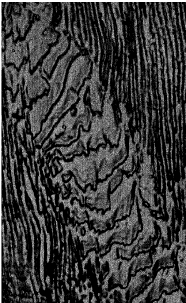
FIG. 24. "SLIPS OF PEARLITE" (By Brandt in the Author's Laboratory.) Alloy No. 8- \omega = 82° - \times 4,500.
