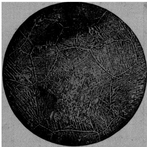
FIG. 26.—WIDMANSTÄTTEN STRUCTURE OF THE ALLOY NO. 8 × 3.
