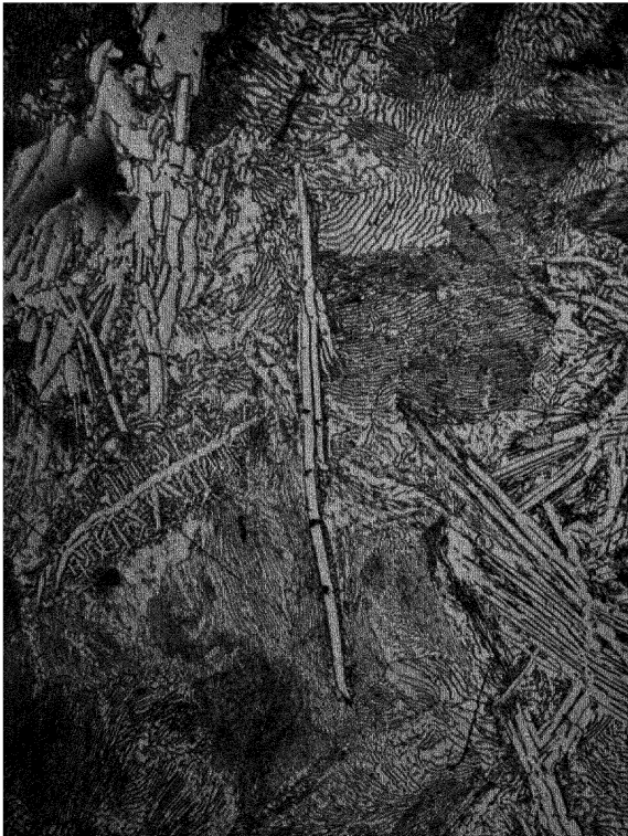
PHOT. 28 - CRACKS ON A CEMENTITE NEEDLE.
