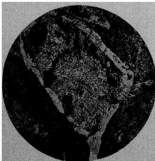
PHOT. 6.—NETWORK STRUCTURE. Alloy No. 5—Ferrite and Pearlite— \times 150 .
