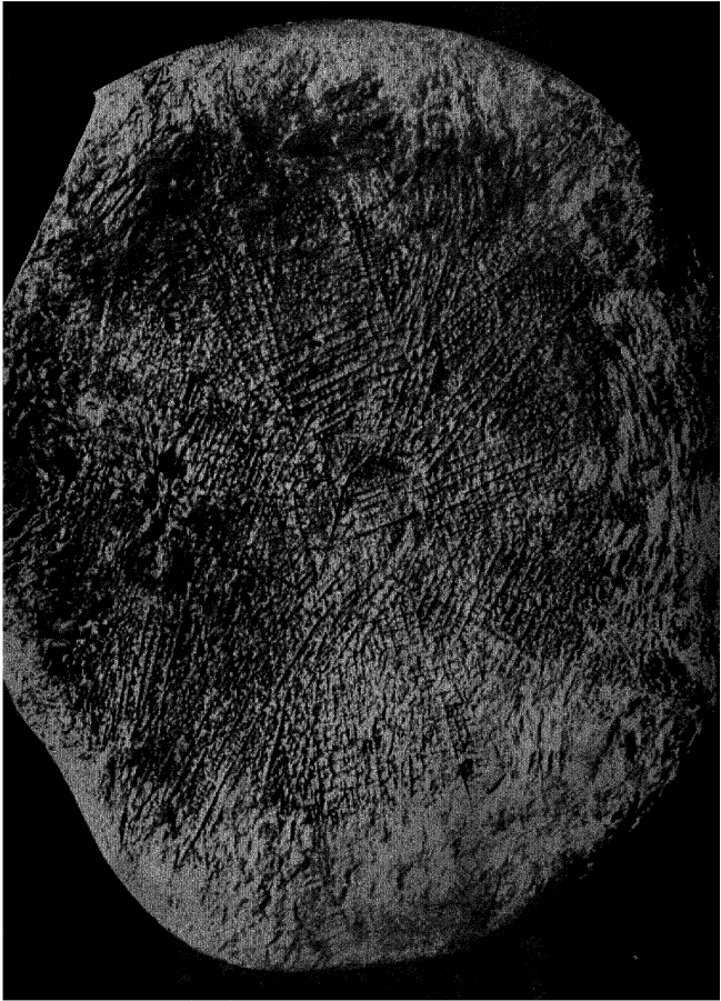
PHOT. 2.—“PRIMARY CRYSTALLISATION.” Alloy No. 2-C = 2.27%— \times 2 .
