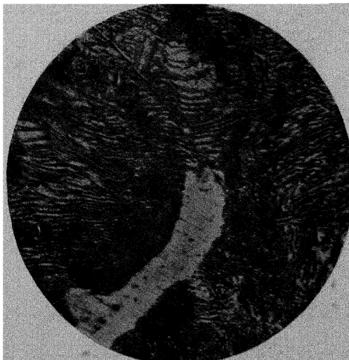
PHOT. 17. Vide PHOT. 16.—THE STRUCTURE OF PEARLITE, × 300.
