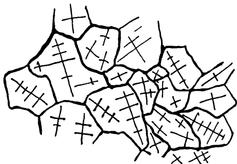
FIG. 14.—PRIMARY DENDRITIC GRAINS. (D. K. Tschernoff, On the Structure of Cast Steel Ingots , fig. 16.)
