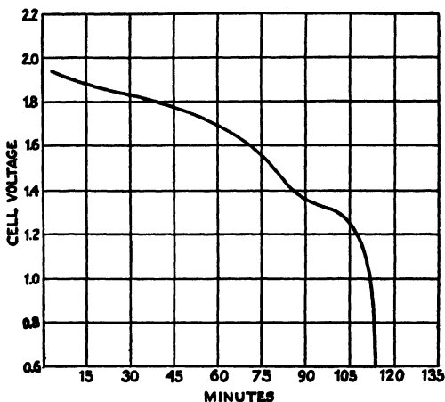
FIG. 36. — Full discharge curve of ribbed Planté plate.
