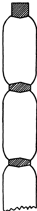
FIG. 86. — Longitudinal and cross sections of a "National" plate.
