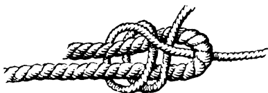
The Double Sheet Bend , for joining ropes of different thicknesses.
