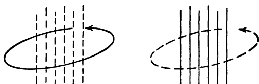
FIG. 47.— A summary of Maxwell's equations for free space: changing electric flux produces linking m.m.f.; changing magnetic flux produces linking e.m.f.
