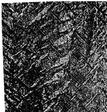
FIG. 81.—Rolled palladium foil saturated with hydrogen electrolytically, etched chromic-nitric acid. \times 150 .
