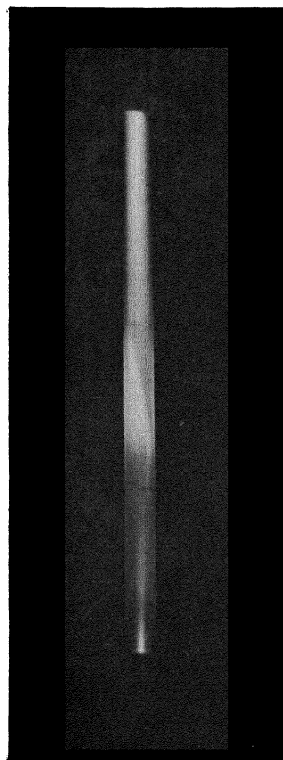
Fig. 41.—Cathode rays attracted by a magnet
