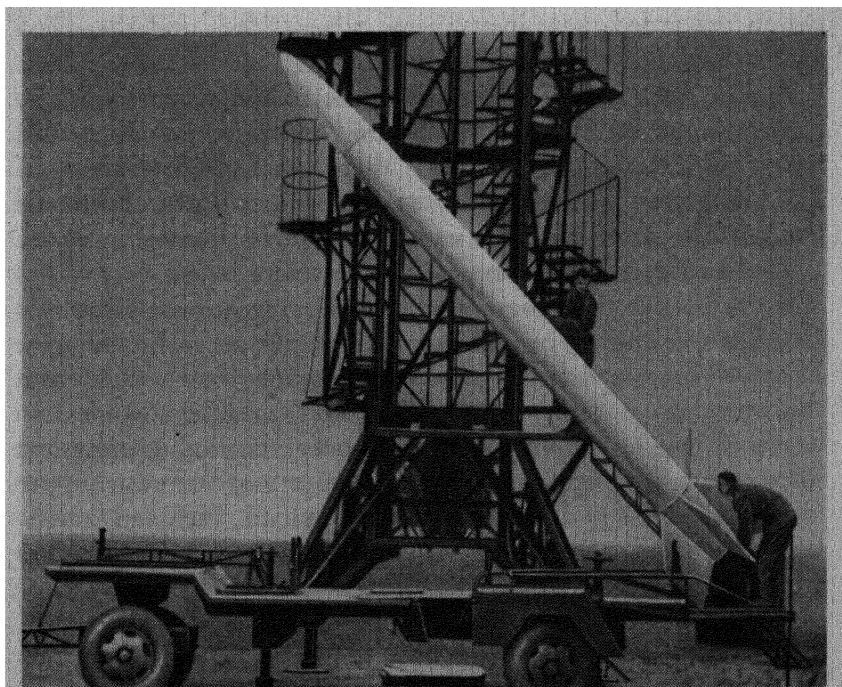
Meteorological rocket on launching rack
