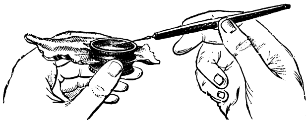
FIG. 346.—DRUM USED TO TEST THE CUTTING-EDGES OF EYE INSTRUMENTS.
