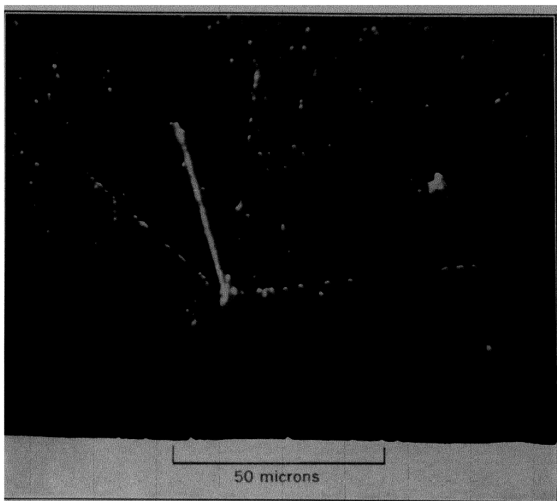
Fig. 63. Cosmic-ray star. In this event one alpha particle and five proton tracks are recorded. If five neutrons were also ejected, the star is consistent with the nuclear evaporation of a N^{14} atom into 1He^4 + 5H^1 + 5n^1 . The total kinetic energy of the fragments is 74 Mev, and, since the binding energy of N^{14} is 76 Mev, the event is consistent with the annihilation of an incident meson of about 300 electron masses.
