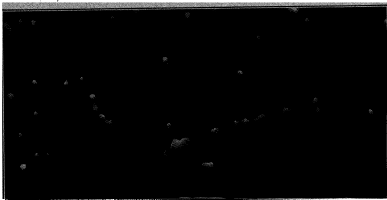
FIG. 44. Comparative grain density in electron and alpha-particle tracks. Eastman NTB emulsion developed by Method II. Dark-field illumination; 2500 \times magnification. The curved electron tracks are more conspicuous when the emulsion is examined visually with a sharply focusing objective. The photomicrograph, taken with a deeply focusing objective in order to depict both events, also includes all the fog grains developed throughout the entire emulsion thickness.
