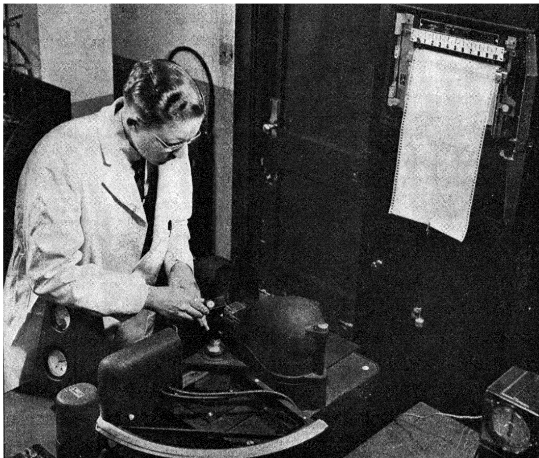
Figure 108. Equipment Used in Determining the Structure of Crystalline Compounds by the Use of X-Rays (Courtesy of Merck and Company;)
