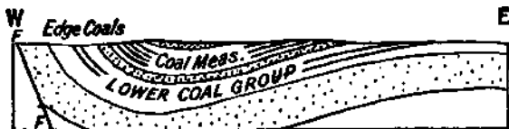
FIG. 174.—A section across the Midlothian Coalfield.
