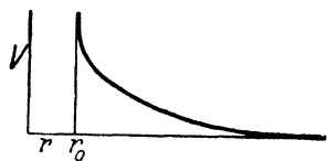
FIG. 8.—Diagrammatic representation of the potential in the interior of and near an atomic nucleus.
