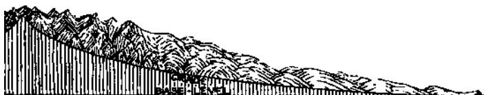
Fig. 53. Longitudinal profile of a graded river, showing the relation of grade to base-level.
