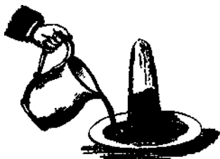
FIG. 9. Porosity of a column of salt
