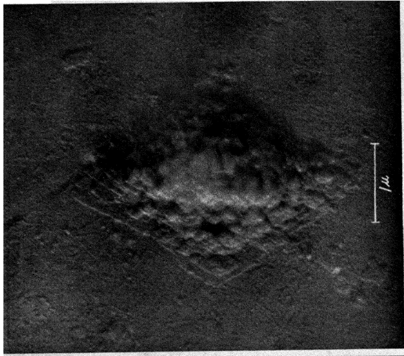
10a and b . Electron microscope photographs of crystallisation of polyethylene. ( 1\mu = \frac{1}{1000} mm.) (See p. 138.)
