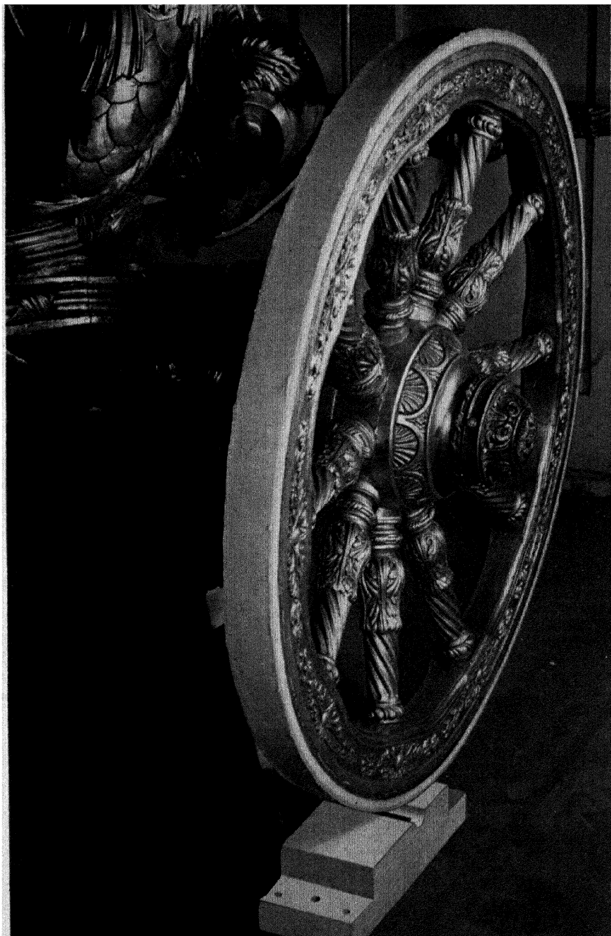
12. The trueing of the wheels of the Royal State Coach by means of synthetic adhesives. (See p. 153.)
