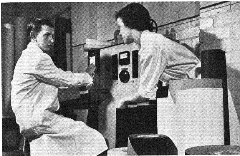
Testing paper for regularity with a Thulium 204 profile unit
