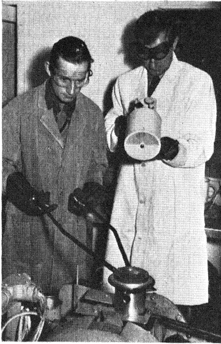
Measuring piston wear
