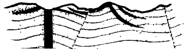
Section across part of Derbyshire, with gently folded and faulted sedimentary rocks, and igneous intrusions
