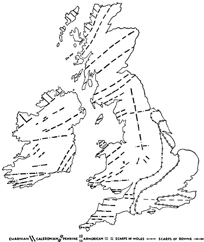
FIG. 311.—Map of the British Isles to show the trend of the folds and other structures resulting from the four main earth-movements. In the case of the Alpine (Wealden) movement, only the scarps produced by denudation of the folds are shown.
