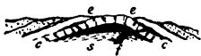
FIG. 124.—Ideal section of a laccolith, showing cover ( c ), sole ( s ), feeder ( f ), and easement dykes and sills ( e ).
