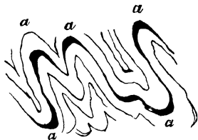
FIG. 72.—Overfolded beds including a seam of coal which has thinned out in the limbs and swelled out in the crests and troughs a a . (B.)
