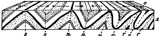
FIG. 70.—Set of folds showing the axial planes. s =symmetrical; n =unsymmetrical; and r =inverted folds.
