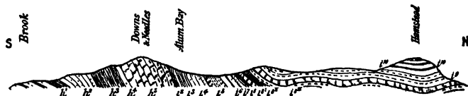
FIG. 256.—Section across the Isle of Wight, h^1 =Wealden strata; h^2 =Lower Greensand; h^3 =Gault; h^4 =Upper Greensand; h^5 =Chalk, i^1 =Woolwich and Reading Beds; i^3 =London Clay; i^4 =Bagshot Beds, i^5 =Bracklesham Beds; i^6 =Barton Clay; i^7 =Upper Bagshot Beds; i^8 =Lower Headon Beds; i^{8'} =Middle Headon Beds; i^{8''} =Upper Headon Beds; i^{8'''} =Osborne Beds; i^9 =Bembridge Beds; i^{10} =Hamstead Beds.
