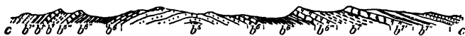
FIG 180.—Section across the anticline of Woolhope, Herefordshire. b^5 =Upper Llandovery Sandstone; b^6 =Woolhope Limestone; b^{6'} =Wenlock Shale; b^{6''} =Wenlock Limestone; b^7 =Lower Ludlow Beds; b^{7'} =Aymestry Limestone; b^{7''} =Upper Ludlow Beds; c =Old Red Sandstone.
