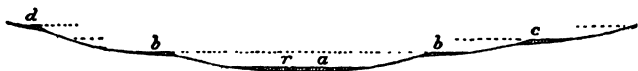
FIG. 56.—Section across a river valley to show the present level of the river a , and the old gravel terraces bb , c , d , the last being the oldest.
