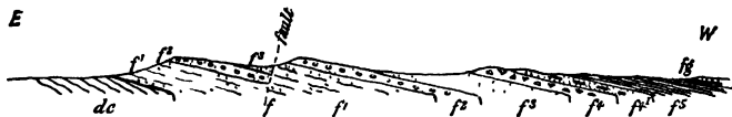
FIG. 216.—Section across the Triassic Rocks of Staffordshire. dc =Carboniferous and Permian Rocks; f 1 =Lower Mottled Sandstone; f 2 =Bunter Pebble-beds; f 3 =Upper Mottled Sandstone; f 4 =Breccia, and f 4' =Building-stone division of the Waterstones; f 5 =New Red Marl; fg =Rhætic Beds.
