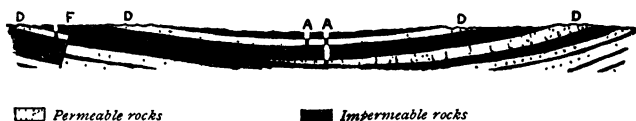
FIG. 305.—Diagram to show the conditions for the formation of an artesian well (A) and a fault spring (F).
